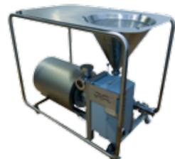
The dimensions of the Hybrid Powder Mixer are H 750 mm x W 826 mm x D 1340 mm. The weight of the complete unit is approximately 280 kg, mounted on wheels for easy handling. The motor is equipped with a VSD (18.5 kW) as standard. The maximum flow generated is 26 m<sup>3</sup>/h. Maximum powder capacity is approximately 3000 kg/h, and the funnel powder volume is 50 l. Media wetted steel parts are in SS 316L (1.4404) and Duplex steel. Funnel, table and frame are in SS 304 (1.4301).
