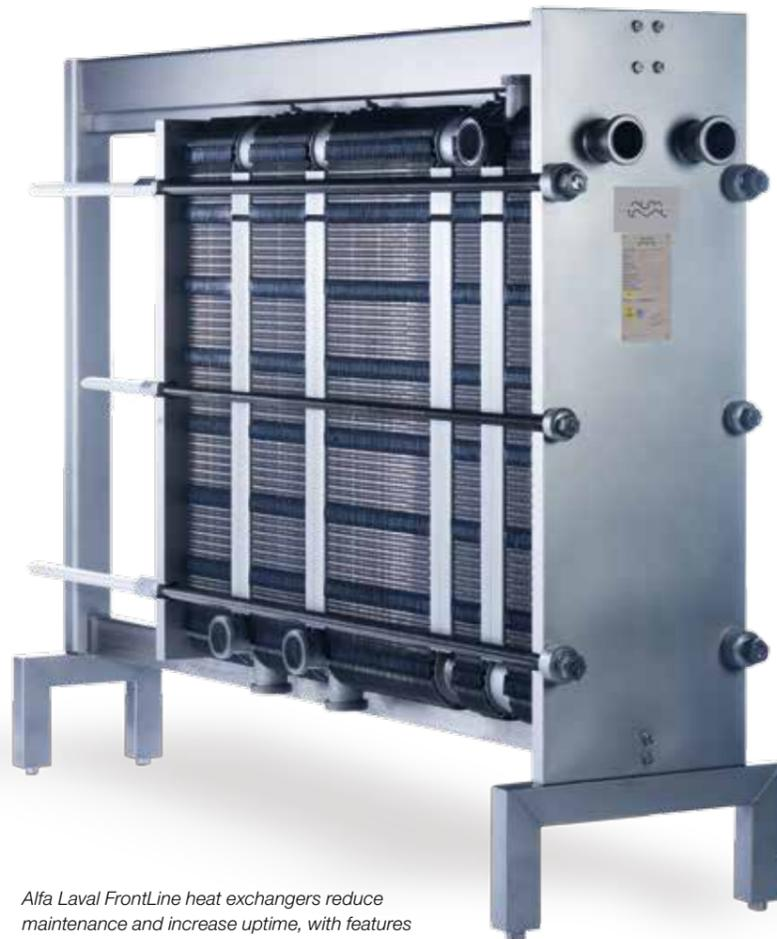
Alfa Laval FrontLine heat exchangers reduce maintenance and increase uptime, with features such as hanging plates, interchangeable corners, and tightening bolts with ball bearings. There is only one gasket size, and re-gasketing can be done without removing the plates.
